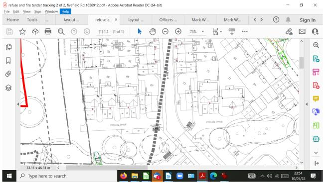
plots 67-70. private drive is 42 m long and has no turning point. The best turning width is 5.5m if the car bays are occupied.
