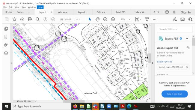
Focus house 314. private drive is 51m long and has no turning point of the required width [16.8m] the max turning space is 5.6m if cars are in the bays.
