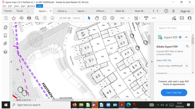
Focus: plot 344 and nearby. The private drive is 108 m long. The max turning space, if the car bays are occupied is 8.4 m (16.8 is min the regs)
